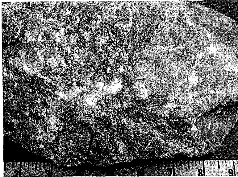
Figure 4. After washing, the Rock Fragment A is shown to be mottled pinkish-beige, gray and white.
